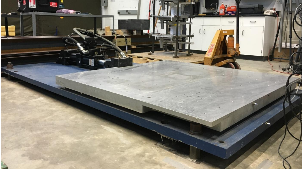
Figure 4.5: Shake table at University of New Hampshire (picture credit Rui Zhang 2016).
