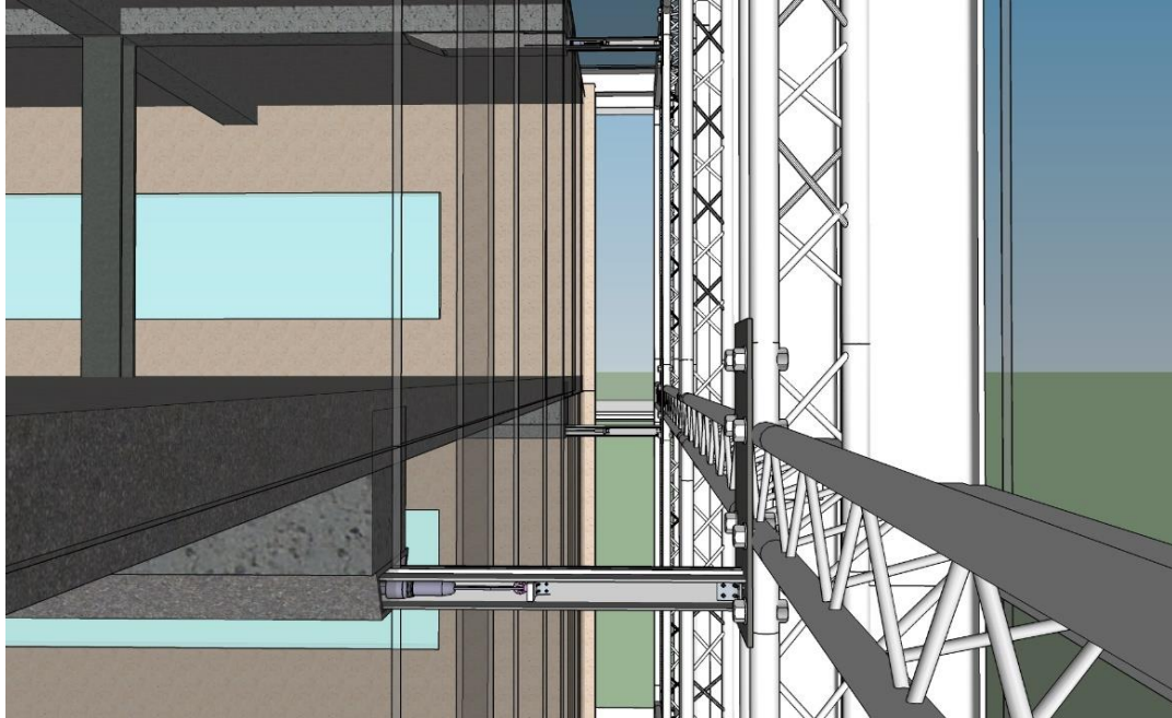
Figure 2.5: Details of the connections between the primary building and the movable façade: the wide flange rail system is attached with bearings, dampers and actuators to allow and control linear motions.
