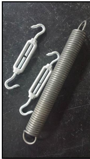
Figure A.2: Spring and turnbuckles used for cross bracing (Picture credit: Kyle Wyatt 2015).
